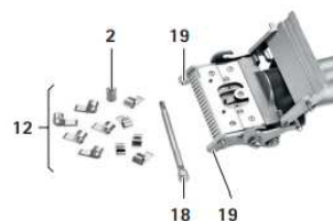
Fig. 13 Flap rod dismantled
